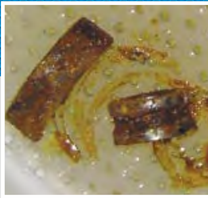
This bearing is 52100 steel. It shows extreme rust in the same test chamber as the Stainless Steel 440C bearing and Cobra Blue treated bearing.
