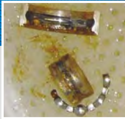
This bearing is Stainless Steel 440C. In this test it showed rust on the races.
