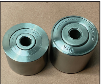
UTA Custom Designed Roller Turn Rolls These units are used over a wide range of temperatures including up to 660°F. 660°F is a continuous rating, CSL660 has a practical limit of 1200°F with very slow degradation over time. Patent US 9,169,080 B2
