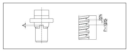
Fig. 18: Safety trap nut SIFA: Dimension "A" for comparison when checking wear
