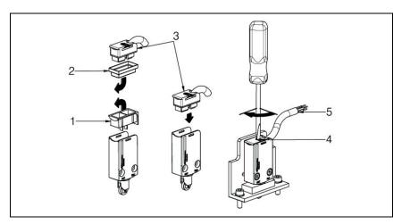
Fig. 12: Fitting the plug connector on the limit switch
