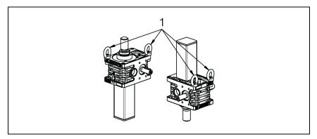
Fig. 5: Fit ring bolts (1) or ring nuts (not supplied)
