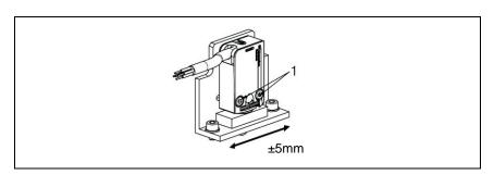
Fig. 15: Adjustment of the limit switch
