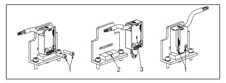
Fig. 14: Turning the cable outlet of the limit switch
