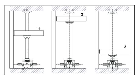
Fig. 17: Correctly aligned screw jack - R version
