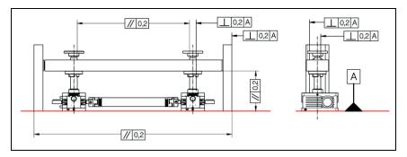
Fig. 7: Flatness, parallelism and angular accuracy
