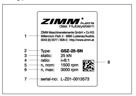
Fig. 2: Example of a rating plate
