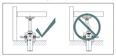
Fig. 6: Side forces on the spindle are not permissible.
