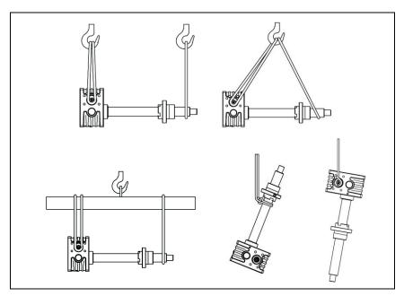
Fig. 4: Examples for transporting the R version
