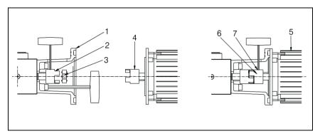
Fig. 11: Installing the motor
