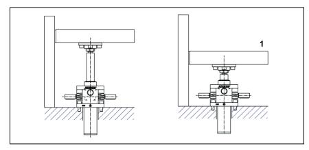
Fig. 16: Correctly aligned screw jack - S version
