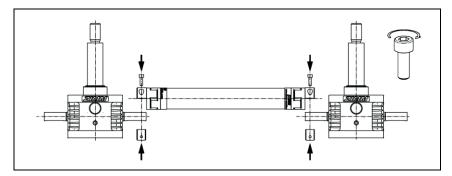
Fig. 10: Installation of connecting shafts
