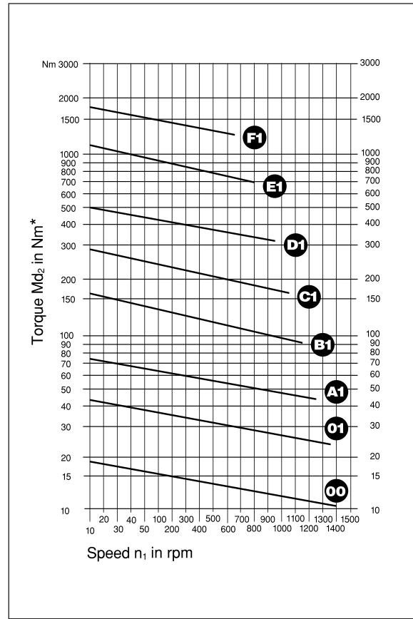
**Selection note:** Lines represent the maximum capacity of each size.
