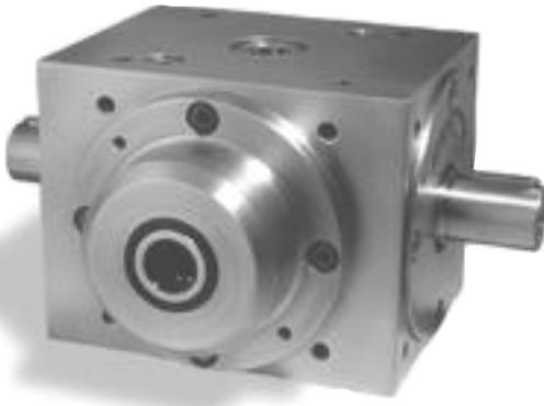
The hollow pinion in the Type HR gearbox contains a keyway, and the hollow pinion in the Type HRZ gearbox contains an involute spline, to facilitate installation directly onto a drive shaft. The torque, speed, and radial load capacity for gearbox types HR and HRZ are equivalent to STANDARD version gearboxes.
