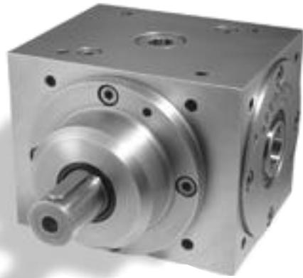
A popular design because it eliminates the need for coupling intersecting shafts or allows for custom shafts to be inserted. Four hollow shaft designs offer increased connection flexibility: key, spline shaft profile, involute spline profile, or shrink disc. The torque, speed, and radial load capacity for type HW gearboxes are equivalent to STANDARD version gearboxes.
