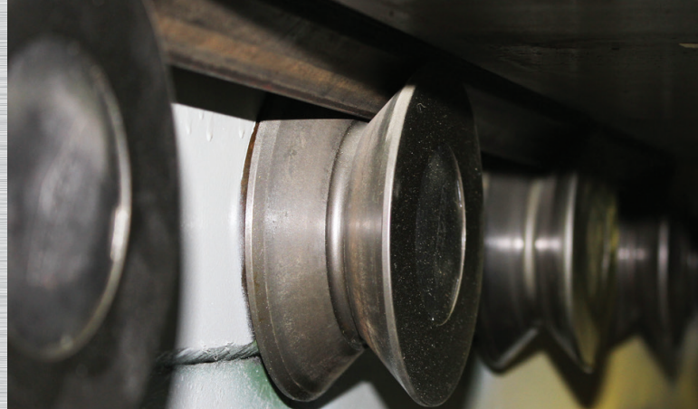
These 180 mm V-groove Load Runners help guide the rack on an oil field hydro tester in the Middle East.
