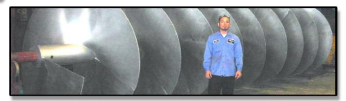
Screw Conveyors can be provided in a variety of sizes ranging from 4" to 36" diameter and as large as 84" diameter with flights up to 2" thick.
